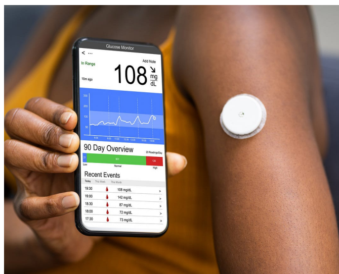
Figure 12.3.1: A CGM on a person's upper arm and its companion phone app, displaying live data and trends.
